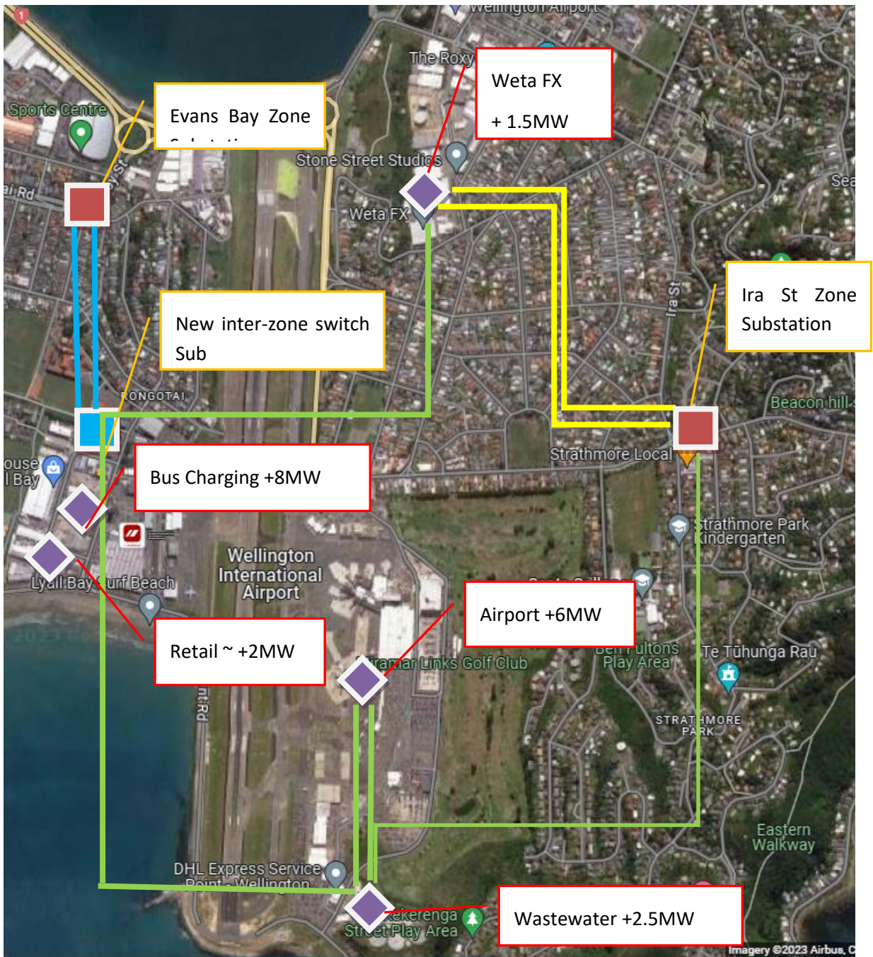
Figure 10 – future network configuration on the Miramar Peninsula
